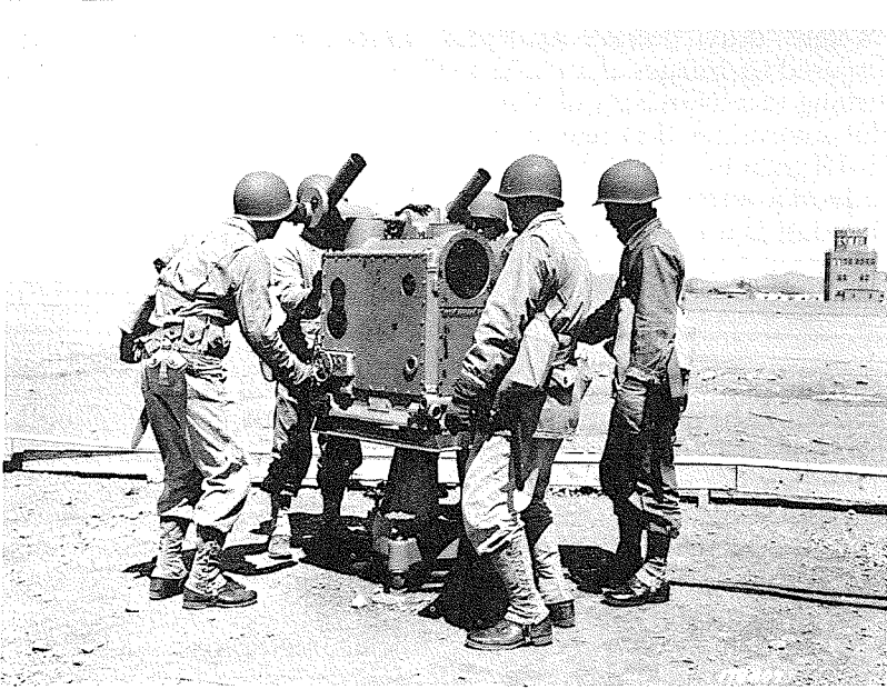
World War II gun directors, such as this one at a Newfoundland base in 1943, did more than help anti-aircraft weapons track enemy planes; they spurred early interest in the idea that machines could be imbued with intelligence.
