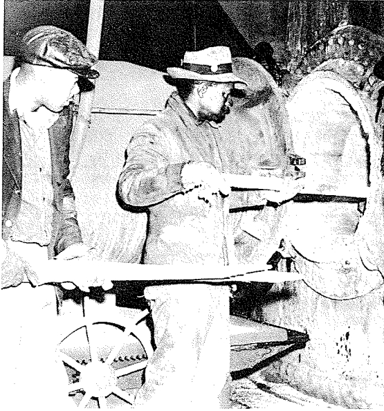
Workmen on the "casting floor" scrape excess hardened metal from the blast furnace.
