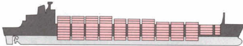
CONTAINERSHIP Dart Atlantic (Brit.) Capacity: 4,500 20-foot containers; 23 knots
