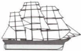
CLIPPER Cutty Sark (Brit.) Cargo capacity: 650 tons (of tea); maximum speed 17.5 knots*
