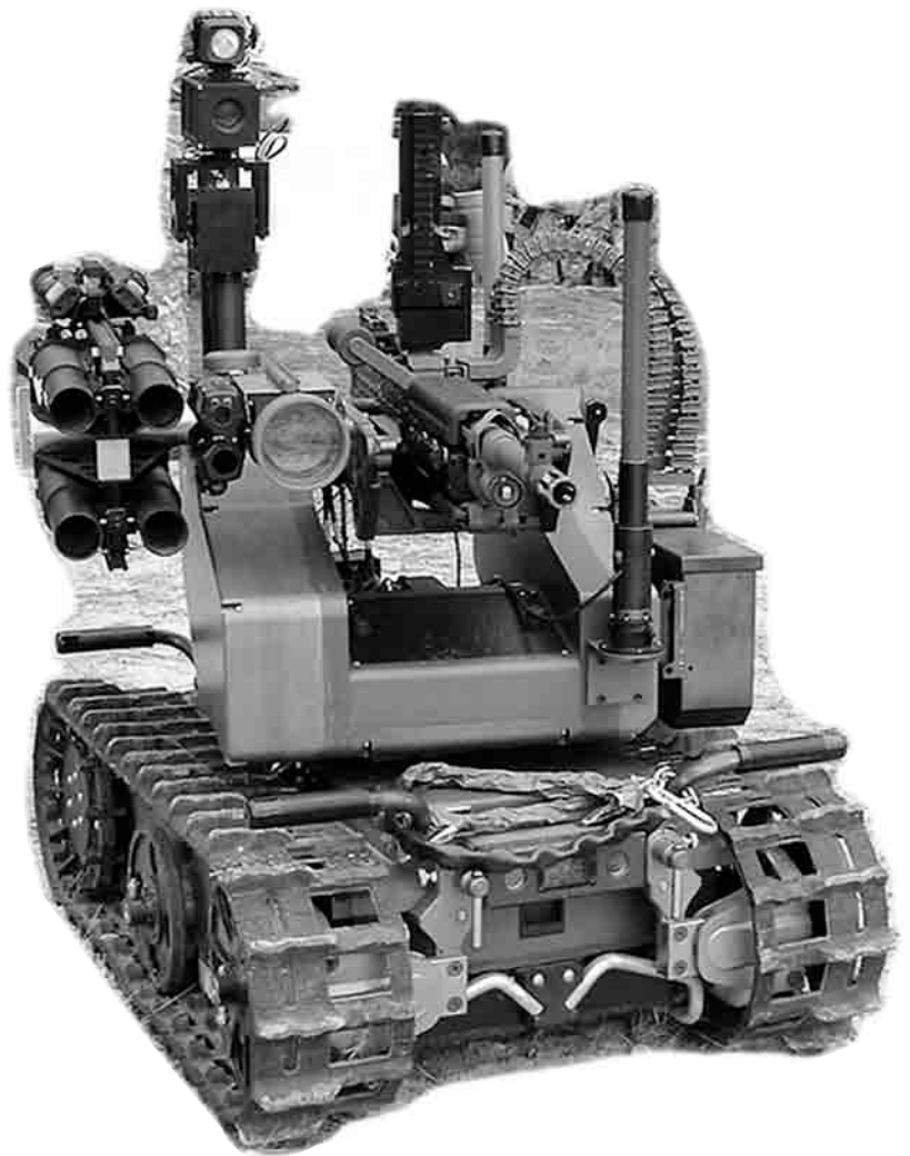
The 350-pound MAARS (Modular Advanced Armed Robotic System), a relative of the TALON, can be fitted with a machine gun, laser, and other weapons.
