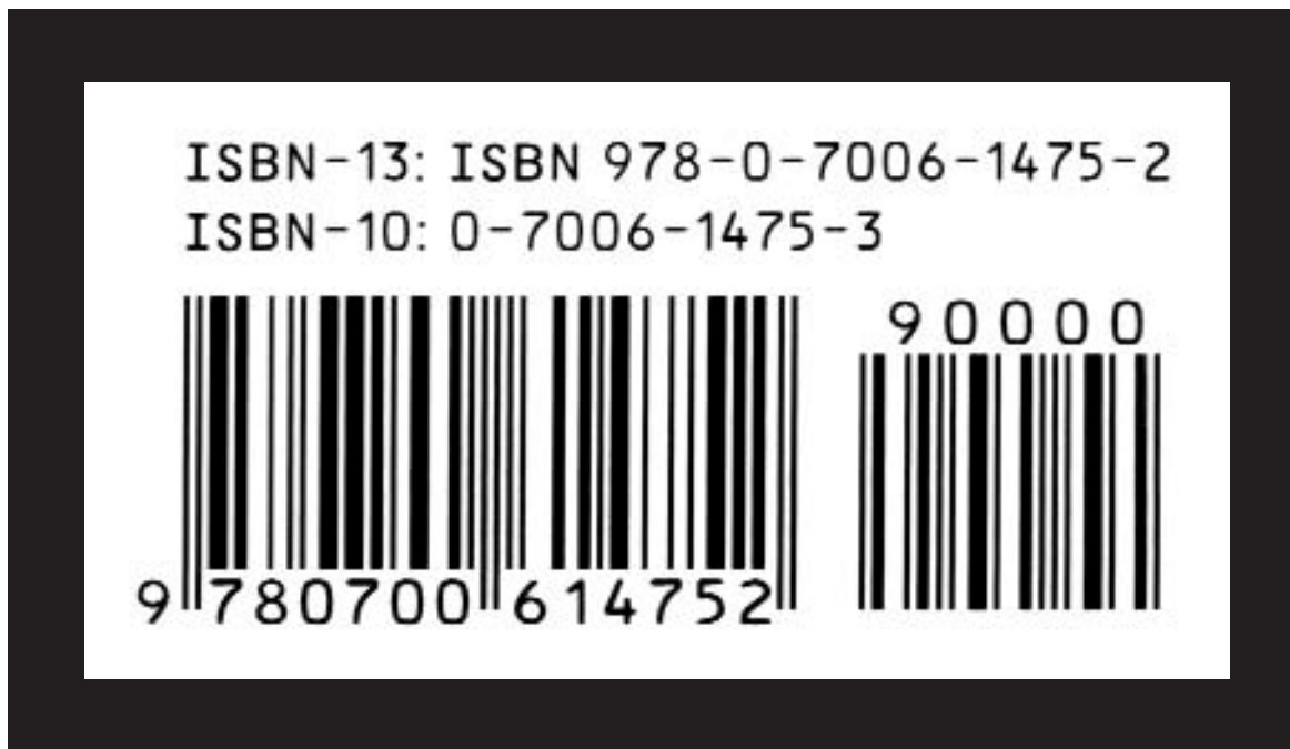
The transitional ISBN format, showing both the old 10-digit and the new 13-digit codes.
